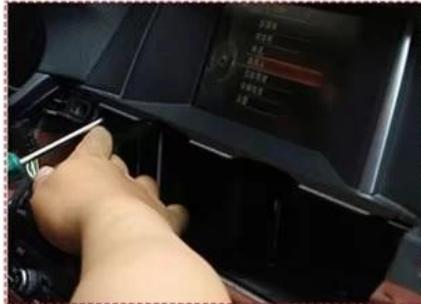
2. Disassembled car original screen
