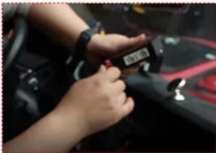
4. Plug the cable with the intelligent box
