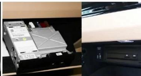
8:Arrange the activator harness and install the CD player back to its original position.
