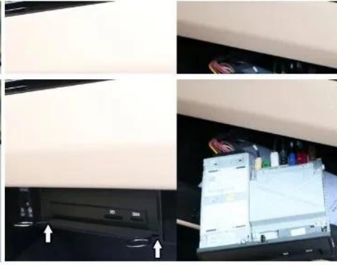
2:Disassembling glove box CD player
