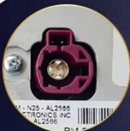
6PIN LVDS Connection
