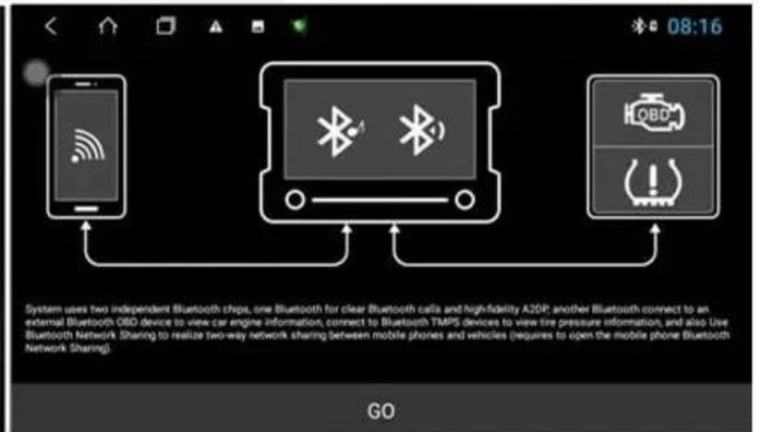
System uses two independent Bluetooth chips, one Bluetooth for clear Bluetooth calls and high-fidelity A2DP; another Bluetooth connect to an external Bluetooth OBD device to view car engine information, connect to Bluetooth TPMS devices to view tire pressure information, and also use Bluetooth Network Sharing to realize two-way network sharing between mobile phones and vehicles (requires to open the mobile phone Bluetooth Network Sharing).
