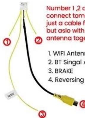
Number 1,2 cable must be connect to model, it's not just a cable for camera but also with wifi antenna together.
