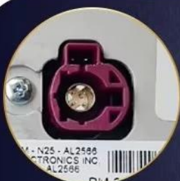
6PIN LVDS Connection
