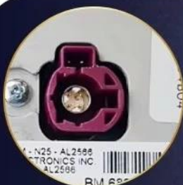
6PIN LVDS Connection
