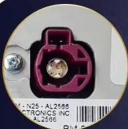
6PIN LVDS Connection
