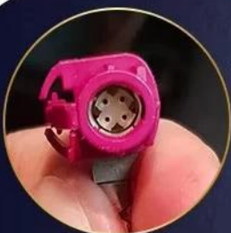
4PIN LVDS Connection
