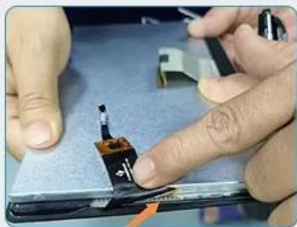
Touch screen cable breakage
