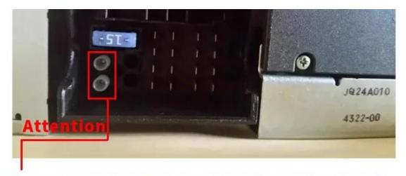
If The original car has the 2interface inside the red box, whichiswith optical fiber, you need to buy an extension cable or fiber box; otherwise there is no sound
