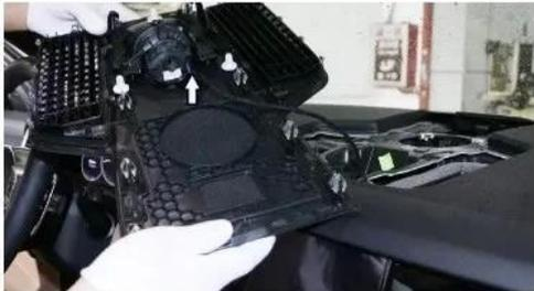
5:Plug in the stopwatch plug of decoder
