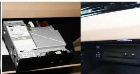
8:Arrange the activator harness and install the CD player back to its original position.
