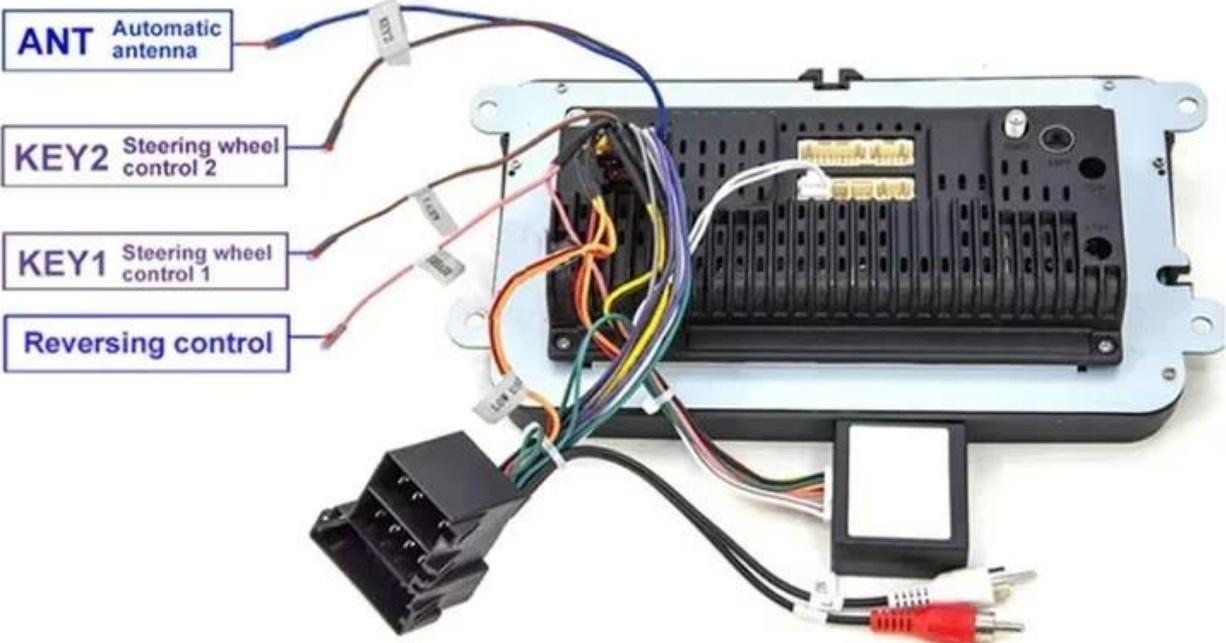
**Installation for low-end model Vw cars Do Not connect the automobile agreement box middle cable connect**
