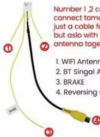
Number 1,2 cable must be connect to model, it's not just a cable for camera but also with wifi antenna together.
