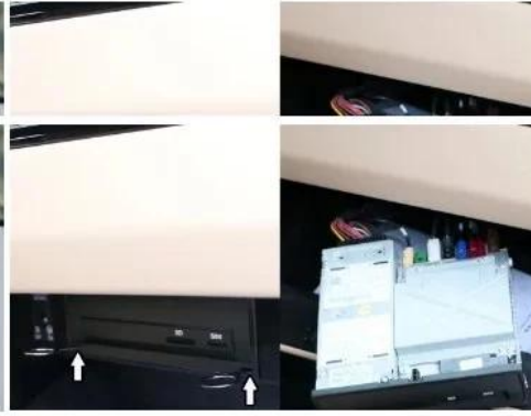
2:Disassembling glove box CD player
