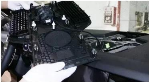
5:Plug in the stopwatch plug of decoder
