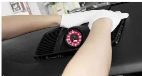
7:Clamp the cover plate from inside to outside
