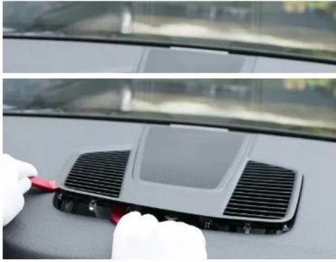
1:Pry off the cover plate of the original vehicle
