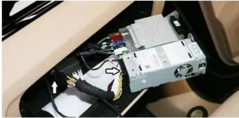
3:The adapter of activator is inserted into the large plug of CD player
