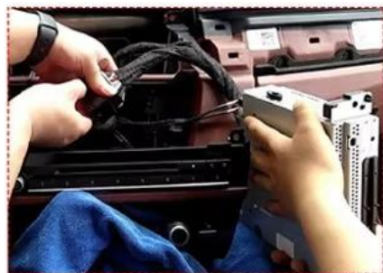
6. Power cable inserted into the original male-female heads
