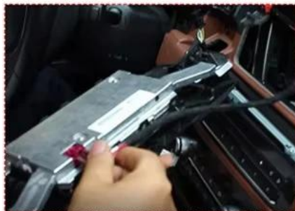
5. Plug LVDS cable with the car screen
