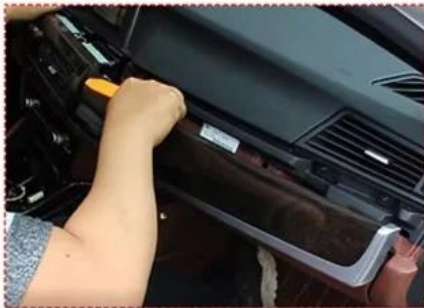
1. Disassembled car decorative panel
