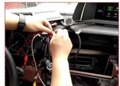
Connect rear camera With the back view LVDS cable
