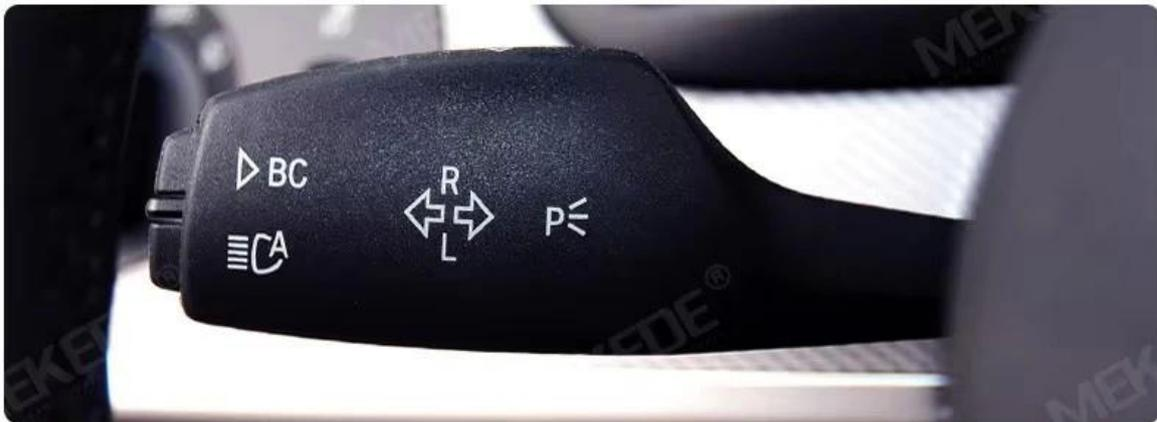
Each time you press the BC key to select a function, long press to confirm and enter the function
