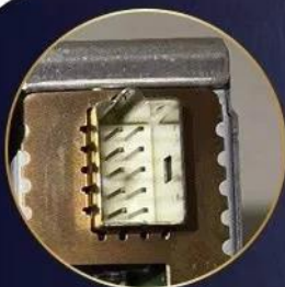
10PIN LVDS Connection
